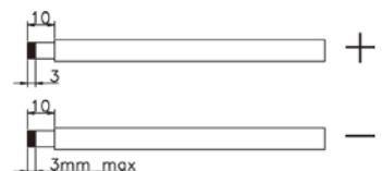
input connector. Connect the negative pole (-) of the connection cable to the negative pole (-) of the photovoltaic input connector.
